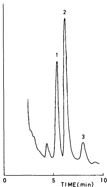
Fig. 2. Gas chromatogram of the methylated neuraminic acids from an oligo-saccharide of the trout egg glycoprotein. 4 % OV-1, 220°. Detection by flame ionization.
